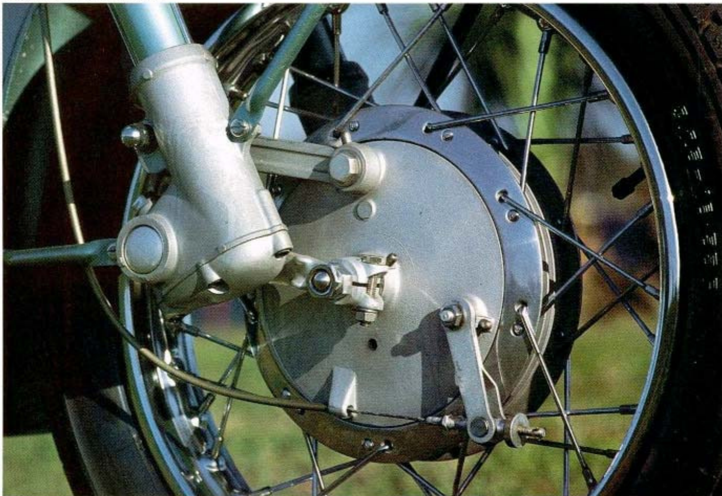
Top: Leading link forks and dual cradle frame were favored by German makers of the day. The space between the wheel and front fender supplied ample room for motion during damping. Below: Detail of the hydraulically-damped leading link front end. The brakes are kept in great shape, as the bike is ridden daily.
