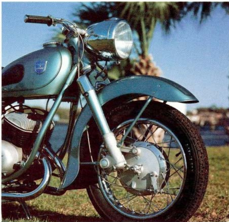
Top: Leading link forks and dual cradle frame were favored by German makers of the day. The space between the wheel and front fender supplied ample room for motion during damping. Below: Detail of the hydraulically-damped leading link front end. The brakes are kept in great shape, as the bike is ridden daily.
