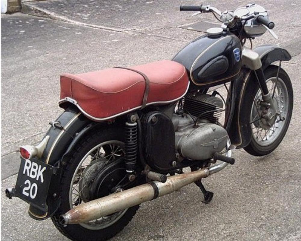
The Favorit is a 250cc twin that was designed as a replacement for the much acclaimed, plunger framed MB250. Released in 1956, the new swinging arm model kicked out 16bhp at 5600rpm giving it a top speed of 73mph, slightly slower than the top of the range, 79mph 18bhp Sprinter model (yes I'm afraid I've got one of those too).
