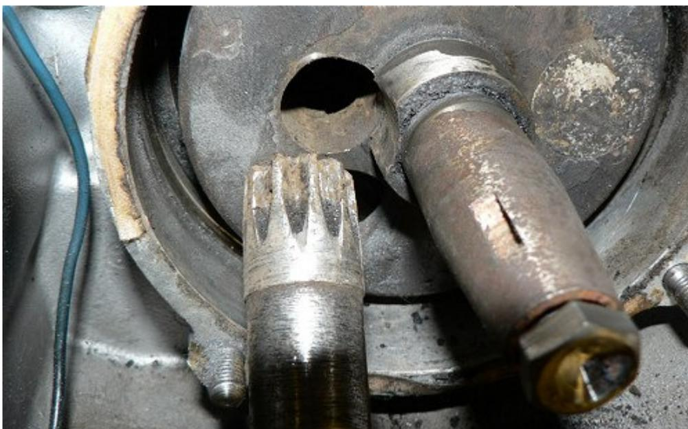
No, it's not as simple as that. You seen the inner bearing race from the offside main bearing remains firmly on the crankshaft, blocking the hole that the Hirth tool is supposed to insert into. You can't get the cranks out to get your best bearing pullers on the race because that race is stopping the job, and that just about takes us back to the beginning of the story.
